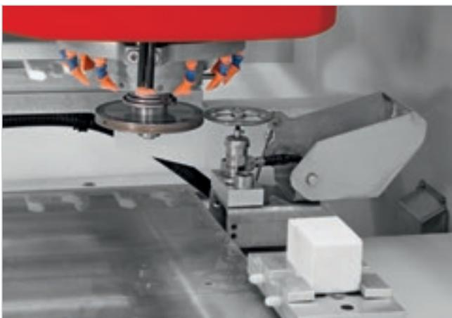
The Master One can be equipped with a **mechanical presetter** that uses a completely automatic system to always provide a quick, simple, precise and updated measurement of the tools during machining operations, avoiding operator error.
