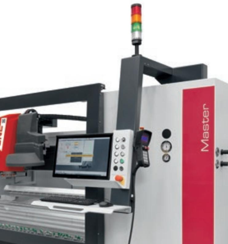
Built-in control panel, with optional touch screen, on the left side of the machine, with the option of installing it on the right side as well.
