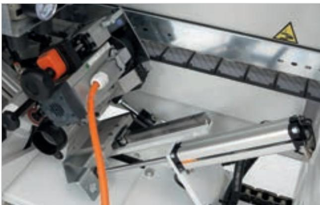
The Multi-purpose corner rounding station with dual motors, forms a radius on both the front/rear and top/bottom edges.
