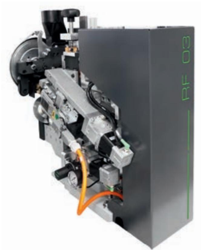
**Fine trimmer unit** trims or cuts the corners on the upper and lower edges of the edgelanding strip applied. Quick and easy adjustment, thanks to 4 controlled axes able to switch between 5 different true profiles and endless other intermediate positions to ensure the highest work quality. Complete with 2 high-frequency 0.65 kW motors (12000 rpm each).
