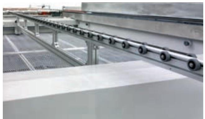
Intermediate bars with automatic positioning function. The positioning of the bar or intermediate bars can be automated; this is recommended when producing small batches.
