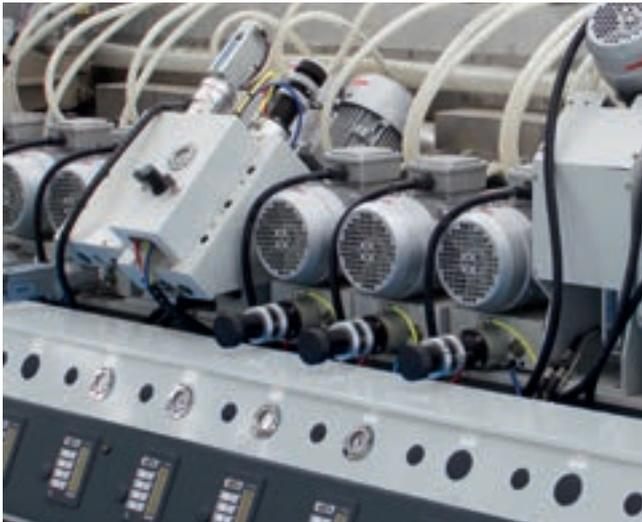
Machine setting times are notably reduced by the proportional valves for automatically managing the pressure on the polishing tools according to the thickness.
