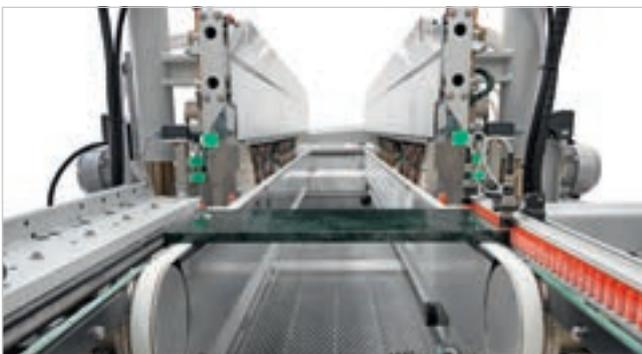
The inlet glass aligning units help the operator to position the glass correctly in the machine, thanks to a proper length of the glass inlet area.
