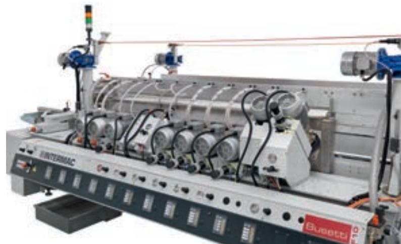
The crosspieces are designed to keep the water away from the spindle movement slides, while their robustness guarantees the utmost reliability and vibration-free grinding.
