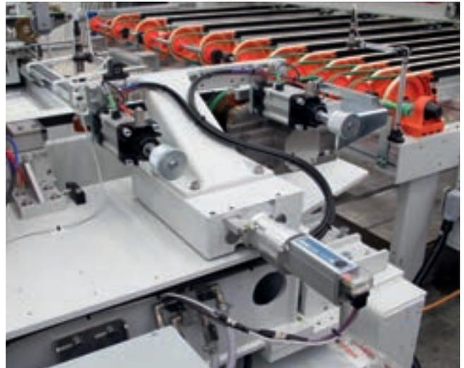
The automatic adjustment of the reference line to remove the glass according to the thickness prevents the operator from intervening manually.
