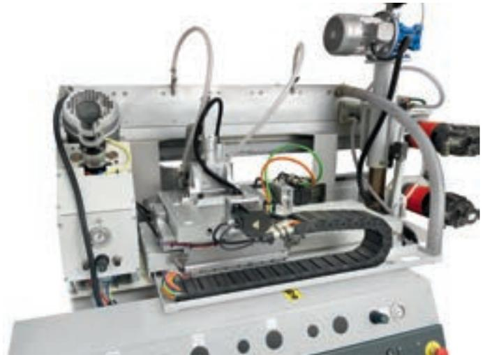
Interpolated axes actioned by brushless motors.
