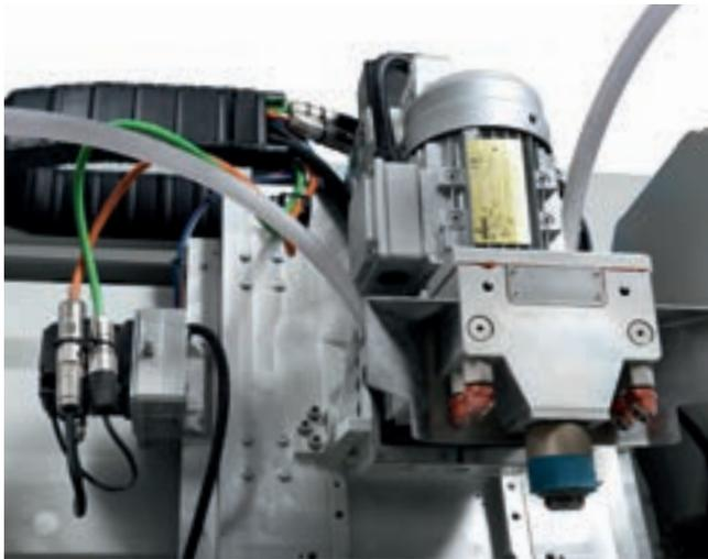
Easy access for the replacement of the grinding wheels, simply by tilting the spindle.
