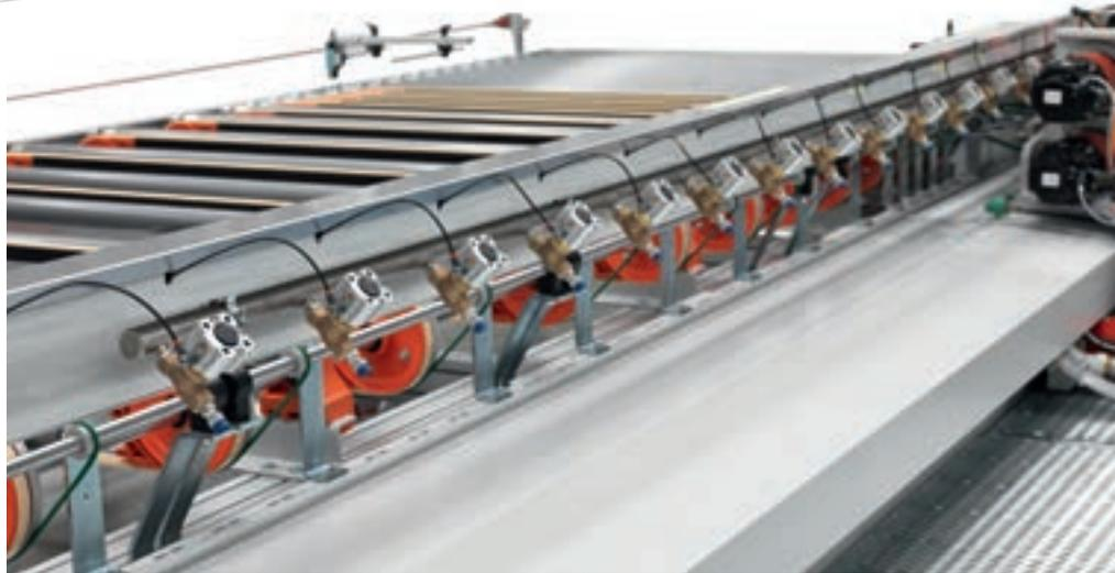
Belt cleaning brush for preventing scratches on the surface of the sheet.
