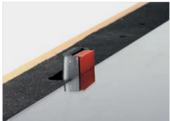
The automatic feet support the sheet while the table is tilting, acting as mechanical sheet aligners when necessary.
