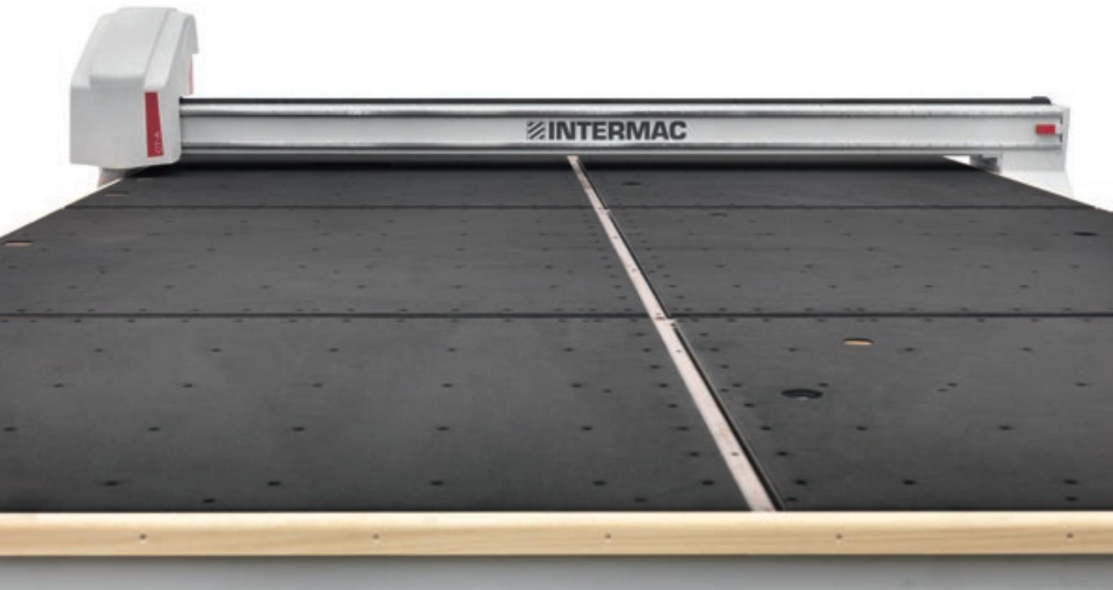
The base of the machine is made from a rigid, rectangular structure onto which ground wood panels are attached, ensuring maximum planarity of the working area, essential for optimal glass grooving and break-out operations.
