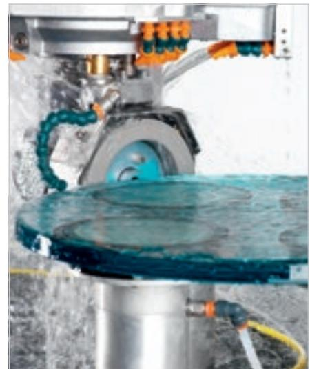
Cup grinding with aggregate.
