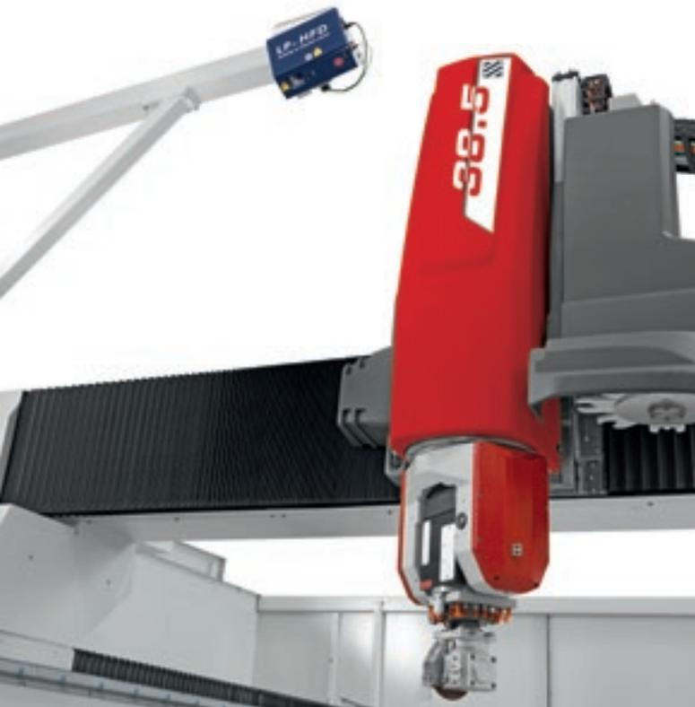
The laser projector is used to make the preparation of the working area quick and easy, reproducing the position of all the suction cups and pieces to be machined on the table and preventing head movements.
