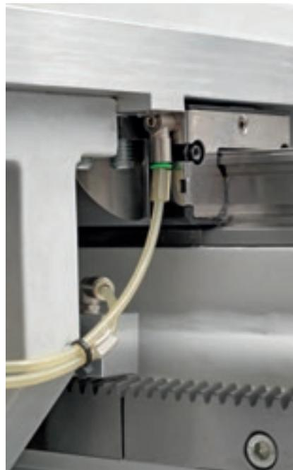
The entire Master range is equipped with an integrated system for the automatic greasing of the movement axes, ensuring constant and precise maintenance every day.
