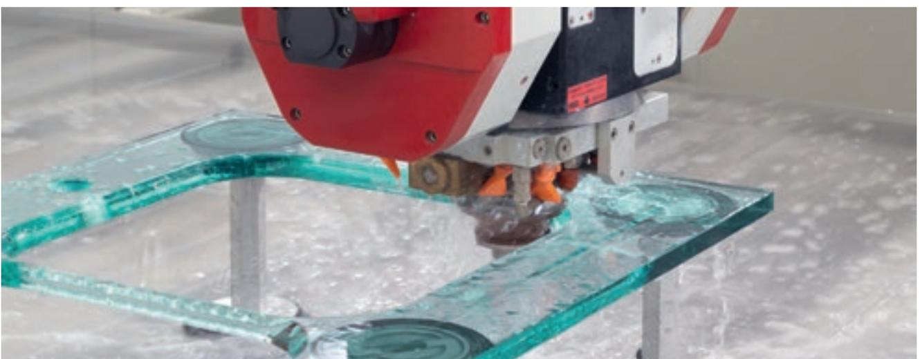
**3 AXIS MACHINING GUARANTEES MAXIMUM RELIABILITY AND ACCURACY FOR THE PRODUCTION OF BATHROOM UNIT TOPS, SHOWER ENCLOSURES AND GLASS FOR DOMESTIC APPLIANCES.**
