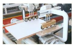
One set of single-side assistance presser ensures the stable work piece feeding, air filled tyres prevent any scraps on panel surface.
