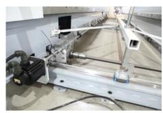
2 ball screw rods on two ends driven by precise servo motor guarantee the adjusting precision ensure two ends move synchronously. Width in between is easy to adjust just by one-click setting.
