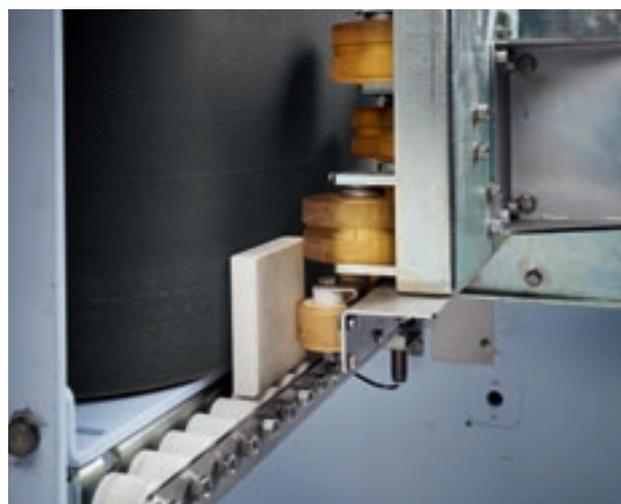
Innovative system with double conveyor belt to guarantee perfect stability, even when working with narrow pieces from 45 mm and heads from 60 mm.
