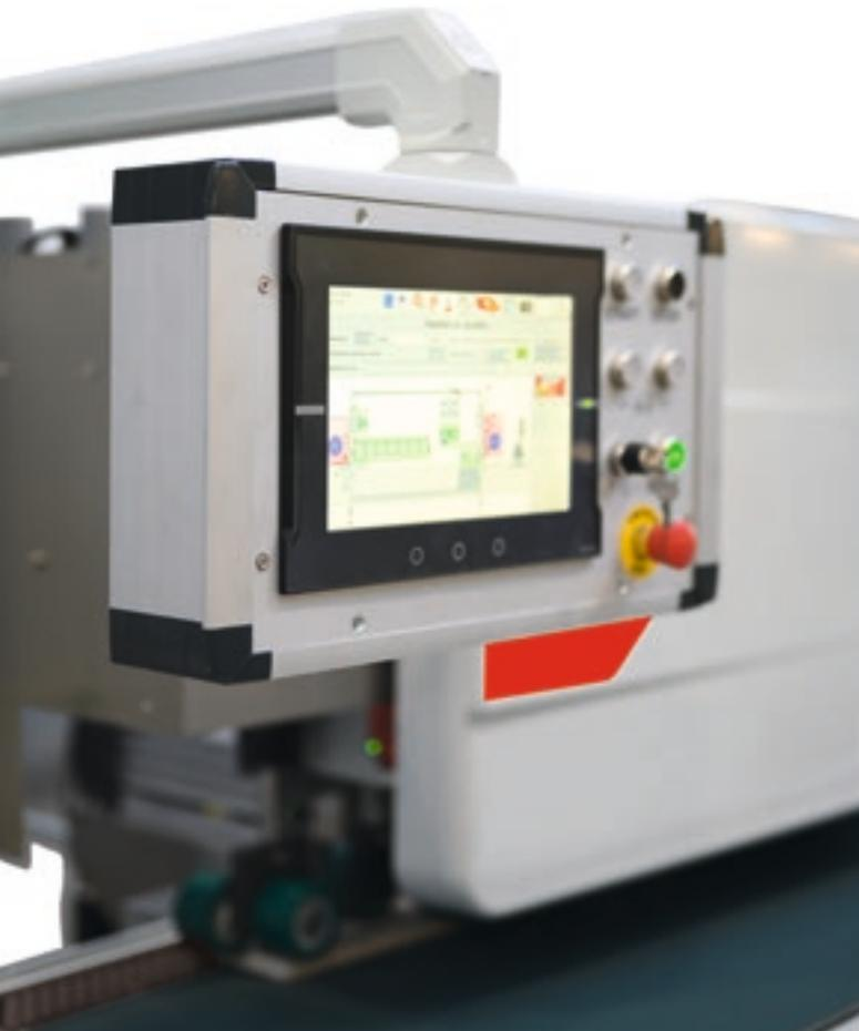
Control panel with swivel arm enables work from different angles and provides maximum visibility and ergonomics for the operator.
