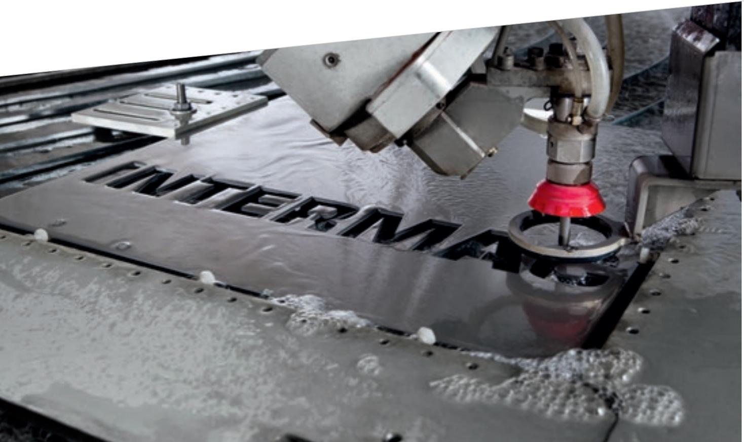
With special applications for variable Z-axis machining operations, this system allows three-dimensional materials to be processed using dedicated software.
