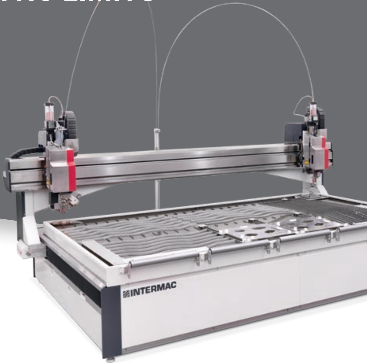
The **Primus Series** is the range of waterjet cutting machines designed to meet the needs of companies looking for maximum versatility. It enables a wide range of materials to be machined, from stone and metal to glass, plastic, ceramics and composite materials.
