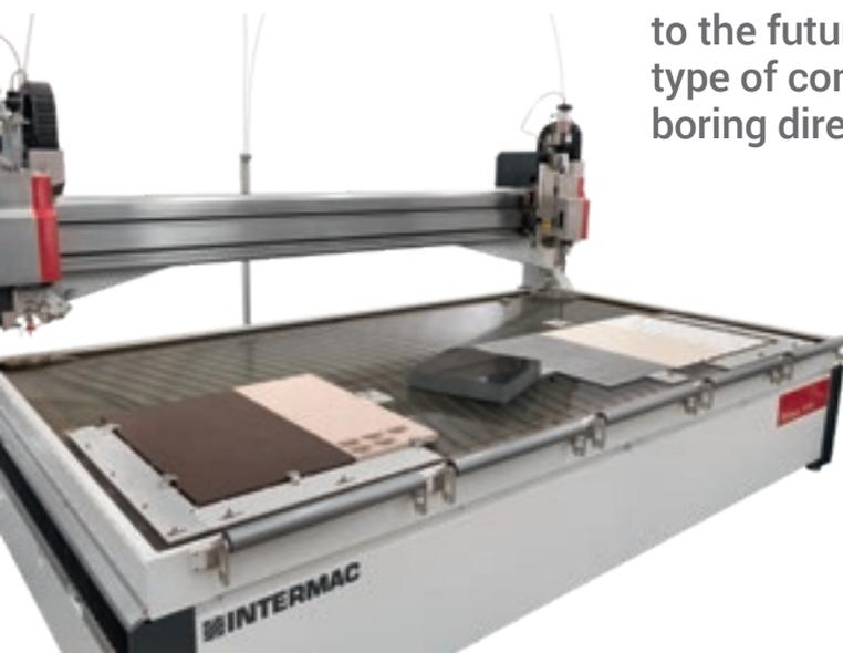
CUTTING FINISH ON GLASS DESIGNED FOR PROCEEDING TO THE TEMPERING PROCESS WITH NO NEED FOR SECONDARY MACHINING OPERATIONS.
