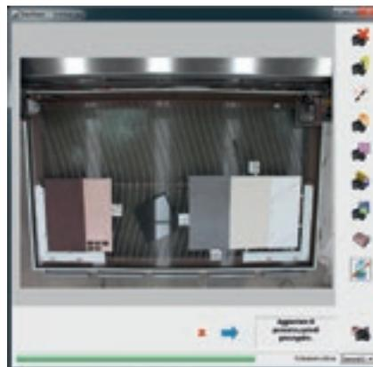
The optional photographic detection system is particularly suitable for open machine operations, where the contours of the natural stone must be followed. Another key advantage lies in the ability to optimise even partially used panels or panels with imperfections, by discarding just the part of the material where the defect is present.
