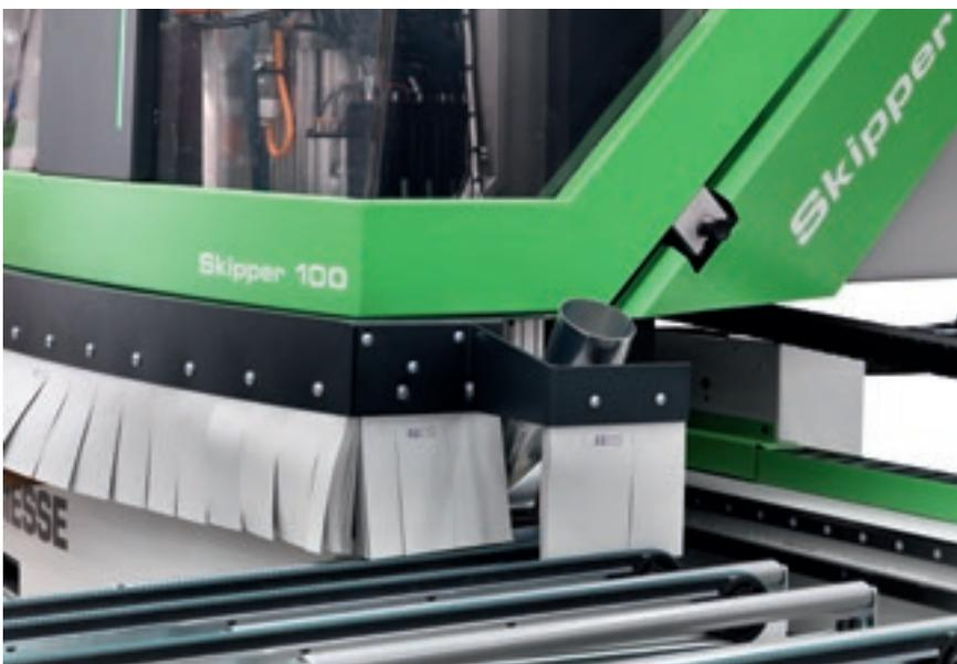
Sound-absorbent covers for the operating sections, with curtain guard barriers (with integrated suction) to protect against dust and waste.
