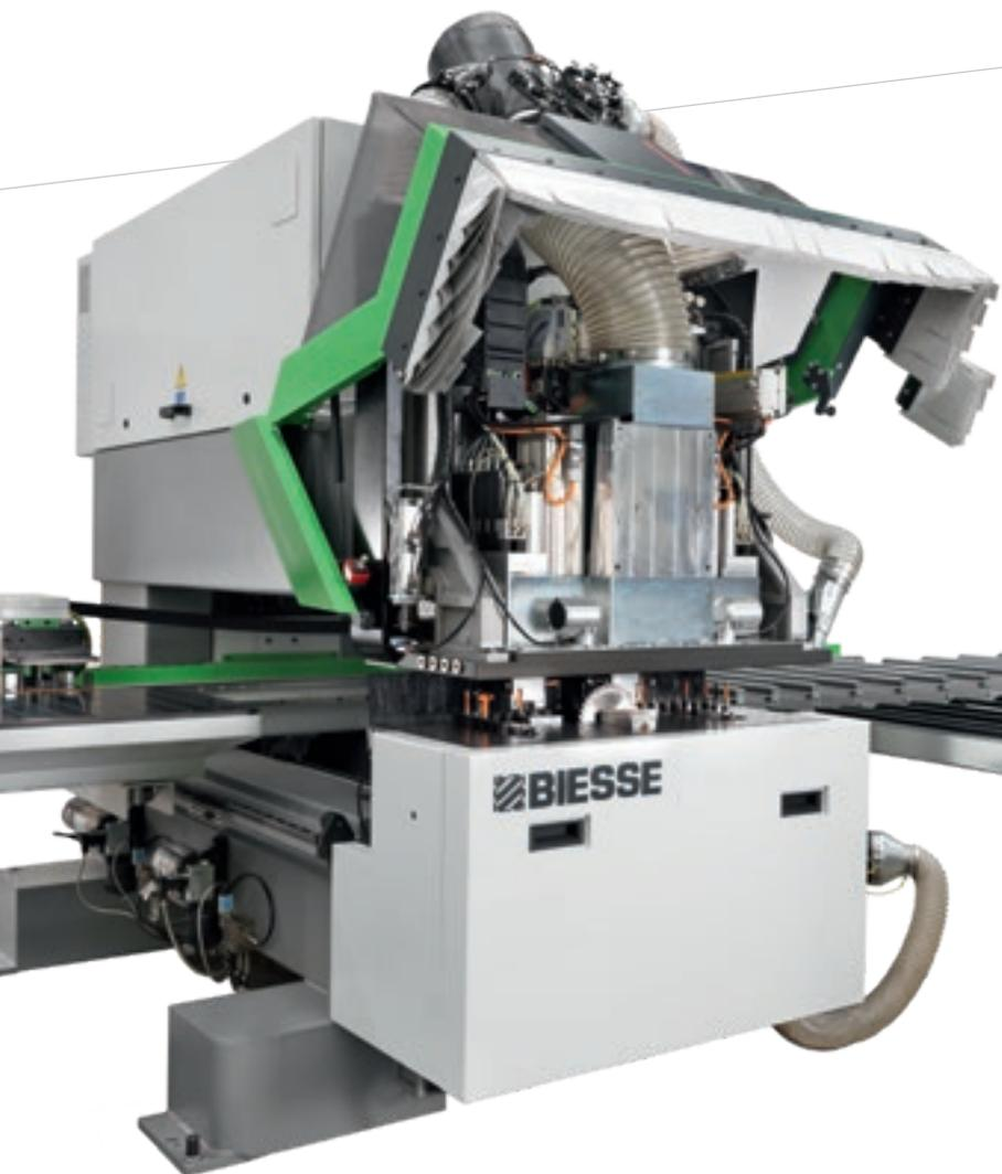
The machining of the machine base on single-positioning processing centres guarantees optimum precision for mechanical operations. The fixed operating sections (and mobile panels) ensure long-term machining accuracy and reliability.
