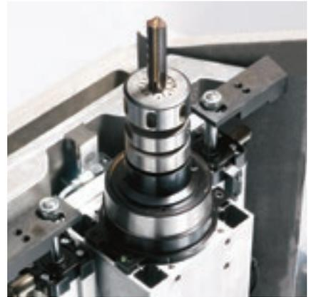
Electrospindles with HSK D-50 coupling.
