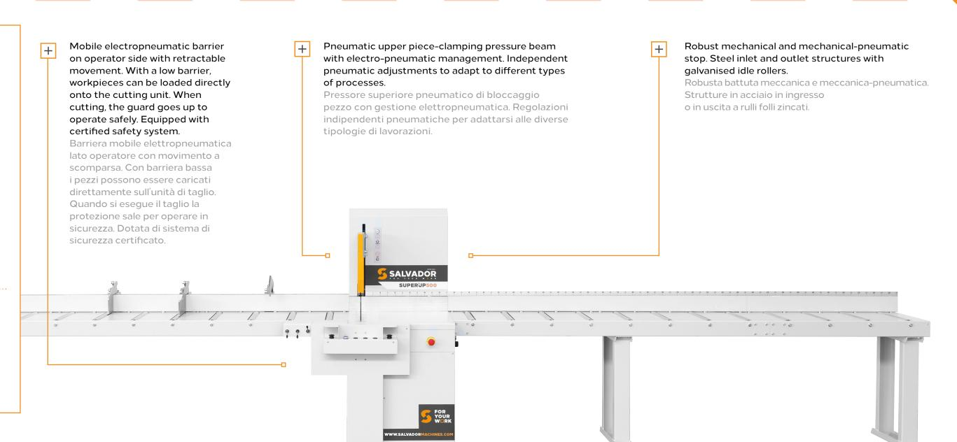
SUPERUP 500 is the new semi-automatic cut-off machine produced by Salvador, an evolution of the historical Classic series. The machine has been improved by designing a sturdier structure, a more accessible and simple adjustment system and a series of innovative options, such as the retractable front guard.
