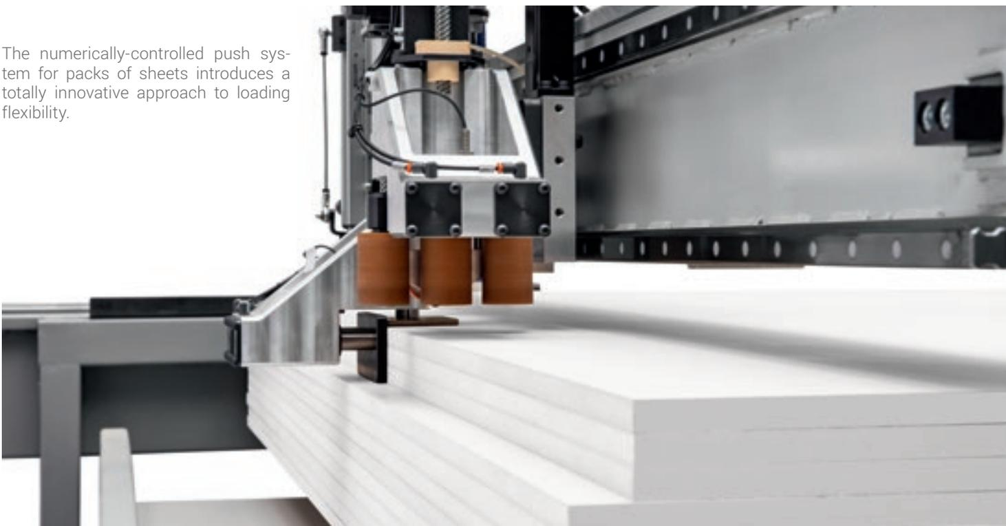
The patented loading system, using collets, allows the loading of books of panels (or highly porous panels) that it would otherwise be impossible to move with the suction cups.
