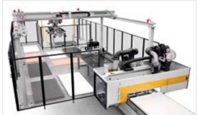
The **Winstore** ensures that the materials to be machined are easily accessible at all times, so it is possible to substantially increase cell productivity compared to manual loading methods using a forklift truck, without frequent stack changes.
